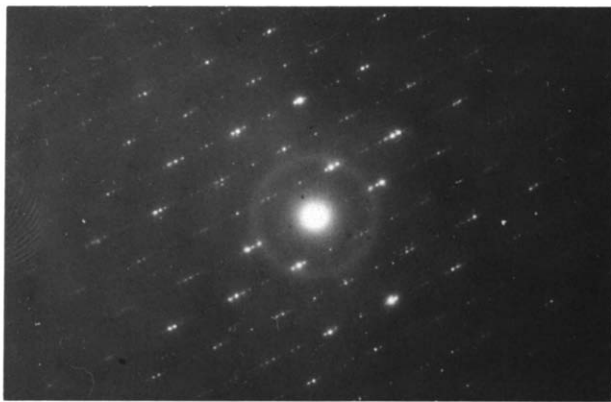
Fig.3. SADP for intergrain space of crystallized material.
